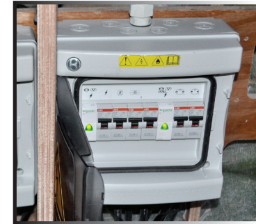
AUTOMATIC BREAKERS FOR ONBOARD APPLIANCES
