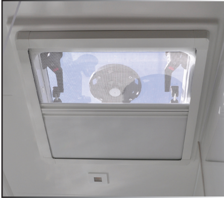
BLIND AND MOSQUITO SCREEN ON DECK HATCH
