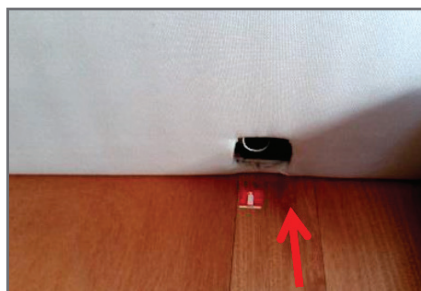
Access to the engine compartment plug
