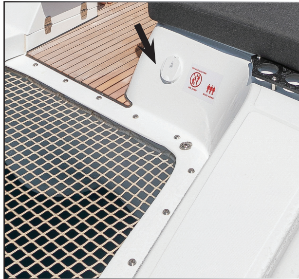
DECK WASHING PUMP CONNECTION
