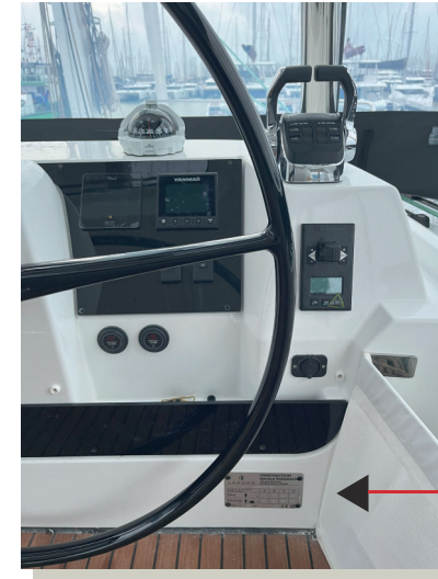
The builder's plate is located at the helm station on the flybridge.
